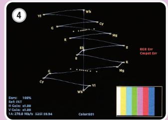
his example shows bowing outward from the center in the upper half of the display. This indicates a timing error in the P'b channel where the P'b signal is leading the luma signal. The transition crosses the third crossnair and indicates a timing error of 74 ns. In the lower half of the display, the green-magenta transition crosses the center mark here is no timing error tween the luma and P'r
