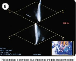
diamond graticule. Note that the trace is offset to the right in the upper diamond. The blue imbalance is caused by an offset in the black level of the blue channel and should be color corrected.
