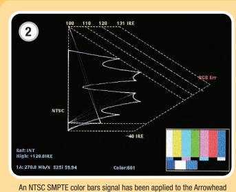
display. In this case, the signal is within the limits of the graticule and will be passed easily through the transmission system. Note that the display indicates that SMPTE color bars are out of gamut within R'G'B' color space.
