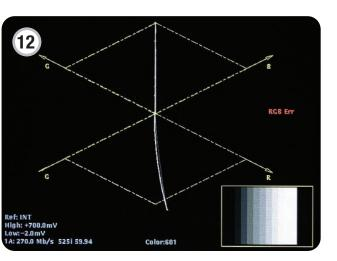
In this case, the camera has a red imbalance that is shown by the deviation of the lower diamond from the vertical axis toward the red axis. The camera should be adjusted to correct for this imbalance.
