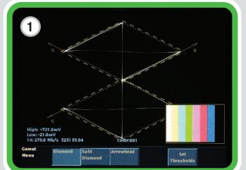
The Tektronix Diamond display using a 100% color bars signal. The 0 to 700 mV signal range of a 100% color bars signal falls exactly within the graticule. The 100% color bars signal is said to be within the gamut of R'G'B' color space.
