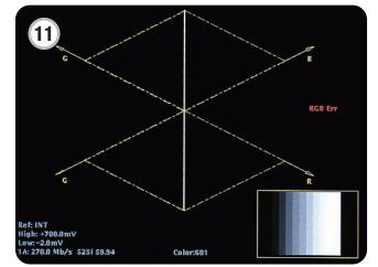
The Diamond display can be an essential tool for simplifying camera balancing. When the value of R'=G'=B', this produces a gray value. A resulting gray scale will therefore produce a vertical line in both upper and lower diamonds, provided the signal is aligned correctly. Any deviation can easily be observed within the Diamond display.
