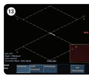
With the lens of the camera capped, the signal should be black and the Diamond display should show a dot at the center of the graticule. In this case, the capping produces a trace along the red axis in the lower diamond, indicating that the red channel has a setup error and should be adjusted until a dot is displayed at the center of the display.
