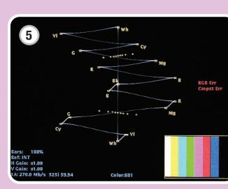
The upper half of this Lightning display shows an error: the traces are not within the graticule boxes. Specifically, this indicates a P'b amplitude error requiring adjustment of the P'b channel gain until each trace fits within the appropriate box. Similarly, if only he lower half of the display was in error, then this would point to a gain error within the P'r channel.
