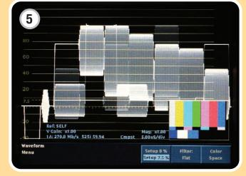
The WFM700 incorporates a pseudo-composite waveform mode that digitally recreates the composite signal waveform from the digital input. This feature allows the operator to visualize the familiar composite signal.
