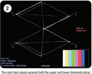
the G' axis. Therefore there is an amplitude error within the green channel and the signal gain should be corrected so that the waveform falls within the graticule. Note that the B' and R' components fall within
