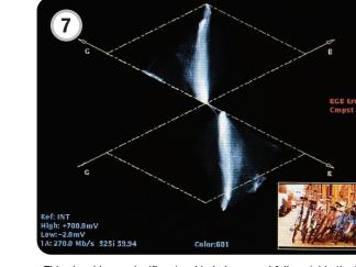
This signal has a significant red imbalance and falls outside the lower diamond graticule. Note also that the trace is offset to the right in the lower diamond. The red imbalance is caused by an offset in the black level of the red channel and should be color corrected.
