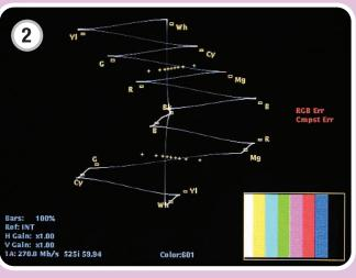
This example shows a luma amplitude error because both the upper and lower traces fall outside the individual graticule boxes. Decrease the amplitude of the luma signal until each component fits within the boxes.
