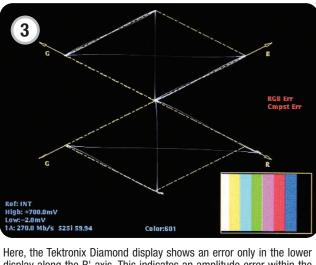
display along the R' axis. This indicates an amplitude error within the red channel. The gain of the red channel should be adjusted to fall within the graticule. Similarly if only the upper waveform falls outside the limits along the B' axis, this would indicate a blue amplitude error.
