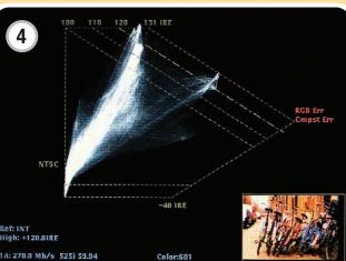
The Arrowhead display can be used for both test signals and live content. In this case, a threshold of 120 IRE has been set and this signal exceeds valid composite NTSC color space. The level of the signal should be adjusted to prevent clipping within NTSC transmission systems.
