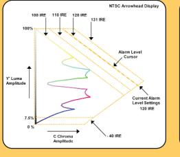
Tektronix developed the Arrowhead display to show out-of-gamut conditions in composite color space, without requiring a composite encoder. The Arrowhead
