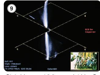
This signal shows an error indicating a green color imbalance. The signal is offset to the left in both upper and lower diamonds indicating a green setup error within the black region. Color correction of the signal is necessary to correct the imbalance.
